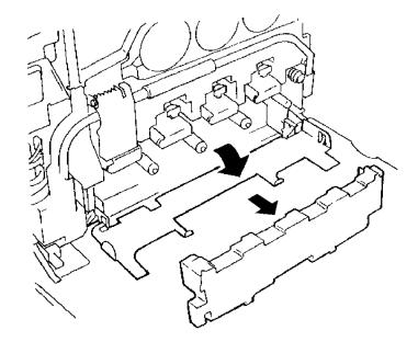
4 Remove the ROS Window Cleaning Tool from its storage area inside the Front Cover.
