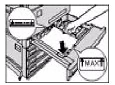
Load the paper into Tray 5 (Bypass) with the preferred printing side down.
