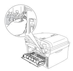
5 Pull the jammed paper out of the fuser unit. If the jammed paper cannot be pulled out easily, push down the blue tab with one hand as you gently pull out the paper with the other hand.
