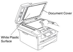
In the ADF unit, clean the white plastic bar and the scanner glass strip under it with isopropyl alcohol on a lint-free cloth.
