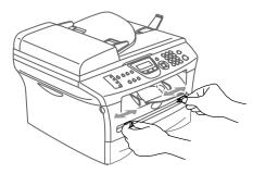
Using both hands put one sheet of paper in the manual feed slot until you feel the front edge of the paper touch the paper feed roller. Let go of the paper when you feel the machine feed the paper in a short distance.
