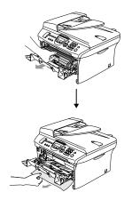
If you can not remove the drum unit and toner cartridge assembly easily, do not use extra force. Instead, lift the scanner cover and use both hands to carefully pull the jammed paper up and out of the output tray opening.
