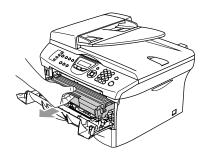
3 Hold down the lock lever on the left and pull the toner cartridge out of the drum unit. Take out the jammed paper if there is any inside the drum unit.
