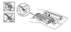
Clean the primary corona wire inside the drum unit by gently sliding the blue tab from right to left several times. Return the blue tab to the Home position (▼) before reinstalling the drum unit and toner cartridge assembly.
