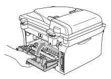
7 Put the drum unit and toner cartridge assembly back into the machine.
